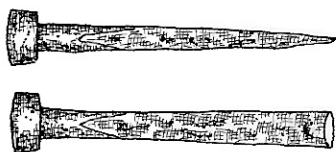
b. Bindhna: the chisel is used for carving and doing wooden joints.
