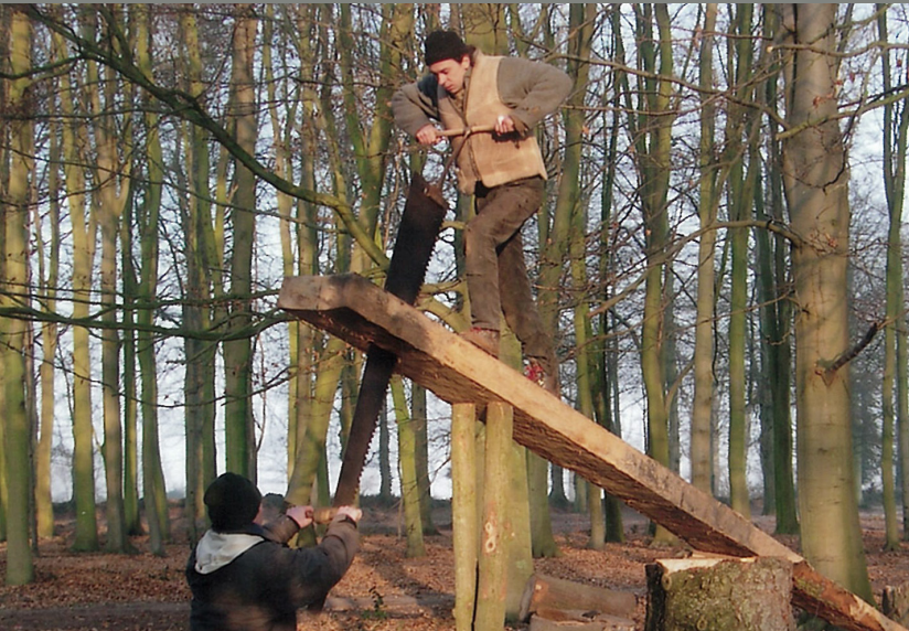
producing quarter sawn beams with a pitsaw
